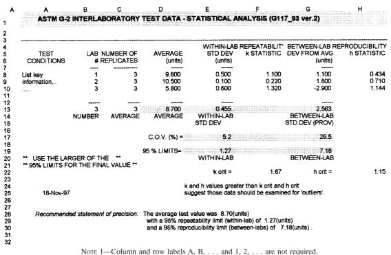
FIG. 1 Example of Recommended Format for Data Analysis
